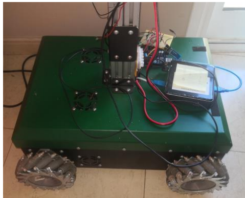
Figure 1. Robotic base employed in the energy consumption experiments.
